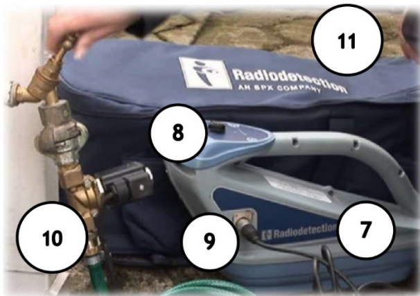
Gambar 7 Anatomi TransOnde Alat Plastic Pipe Locator RD500
